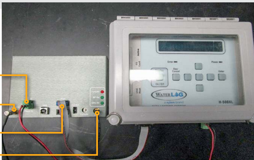
Figure 2: H-2221 Satellite Transmitter connected to an XL Data Logger
